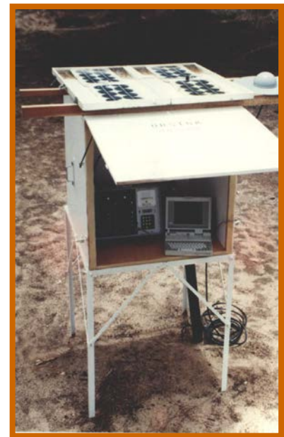
Figure 2 : a magneto-telluric station This station measures the three components of the Earth's magnetic field (X,Y,Z) and the two components of the Telluric electric field 'Ex, Ey).
